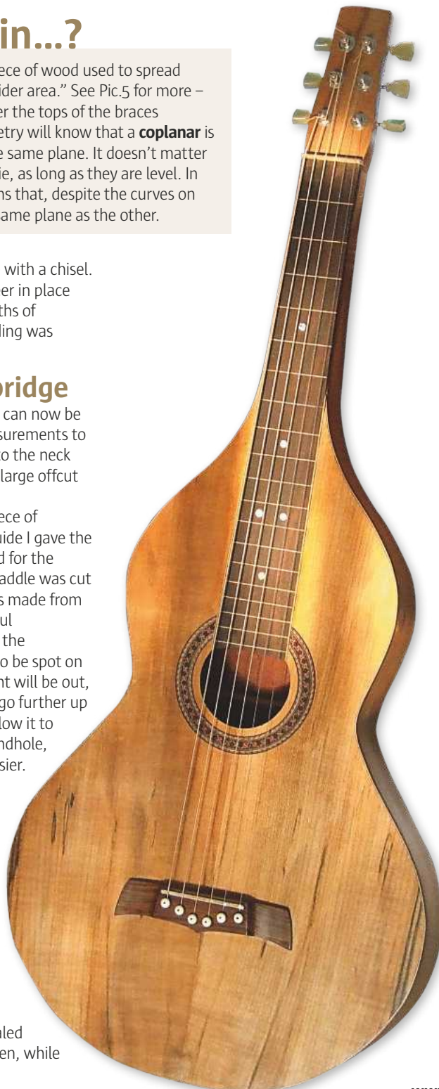
▲ Pic.28 The coat of oil was applied and wiped off after five minutes. Six coats of shellac were then applied
